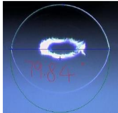
Ordinary IPC Contact Angle (79.84°) of Water Droplet
